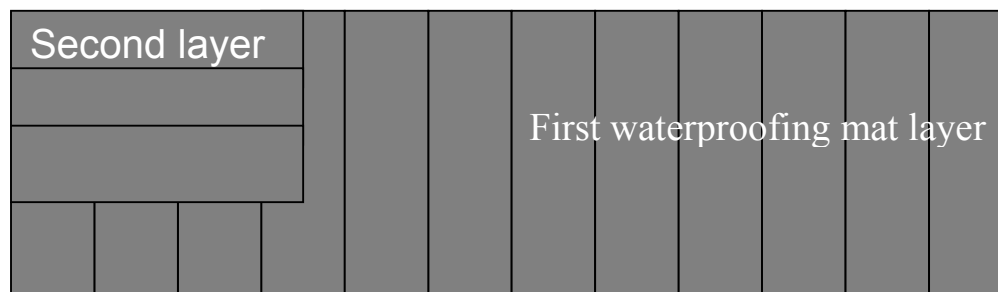
Figure 1. The principle of the waterproofing layout.
